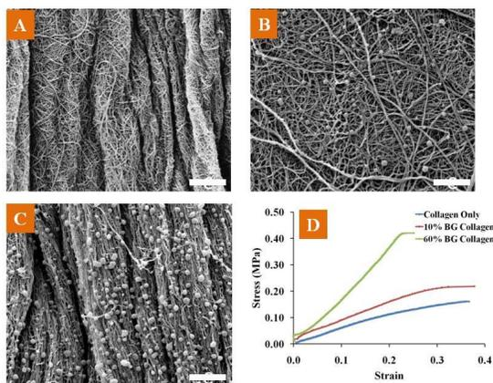
**Figure 1:** (A-C) SEM images for collagen only (A), 10% BG (B) and 60% BG (C) ELAC fibers. Scale bar = 2  $\mu$ m. (D) Stress vs. strain curve for mechanical assessment of nBG incorporated ELAC fibers.
